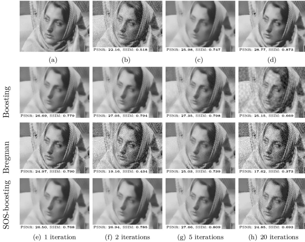
Figure 16. (a) Image x_0 with moderate patch redundancy. (b) Noisy version y = x_0 + w . (c) Nonlocal means \hat{x}(y) with h = 5.5 . (d) Covariant refitting \mathcal{R}_{\hat{x}}(y) . (e)–(h) From top to bottom, boosting [48, 4], Bregman iterations [5], and SOS-boosting [38] at, respectively, 1, 2, 5, and 20 iterations.
