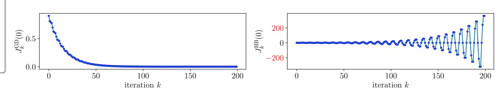
Behavior of automatic differentiation for first-order methods on a piecewise quadratic function. (Left) Stability of the propagation of derivatives for the fixed step-size gradient descent. (Right) Instability of the propagation of Heavy-Ball initialized.
